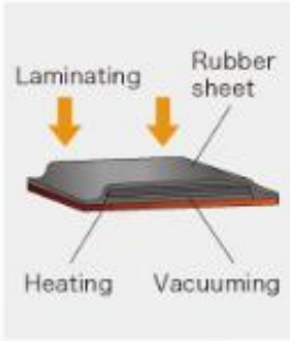
Vacuuming/ Bonding technology
