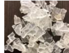
Glass from broken solar panel
